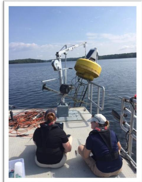
Maintain real-time water quality monitoring buoy in Lower Bay and continue refinement of data interface and data transmission
