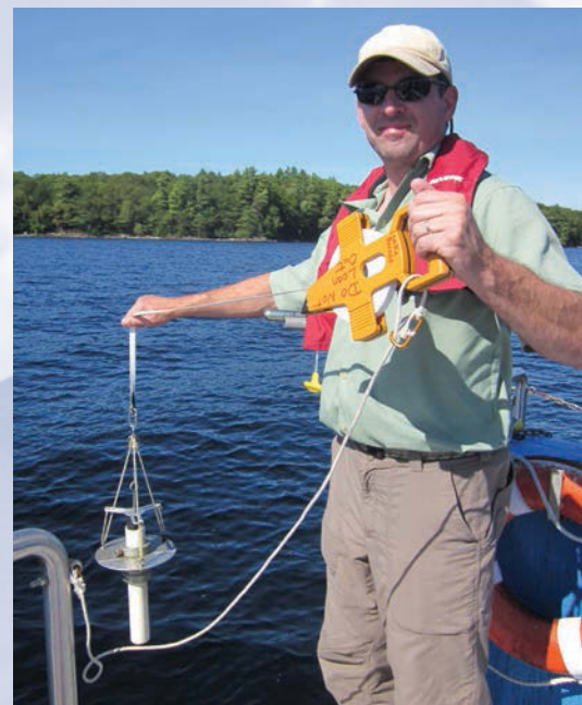
Water Resources Specialist Nate Whalen gets ready to collect a sediment sample for the sediment chemistry study
