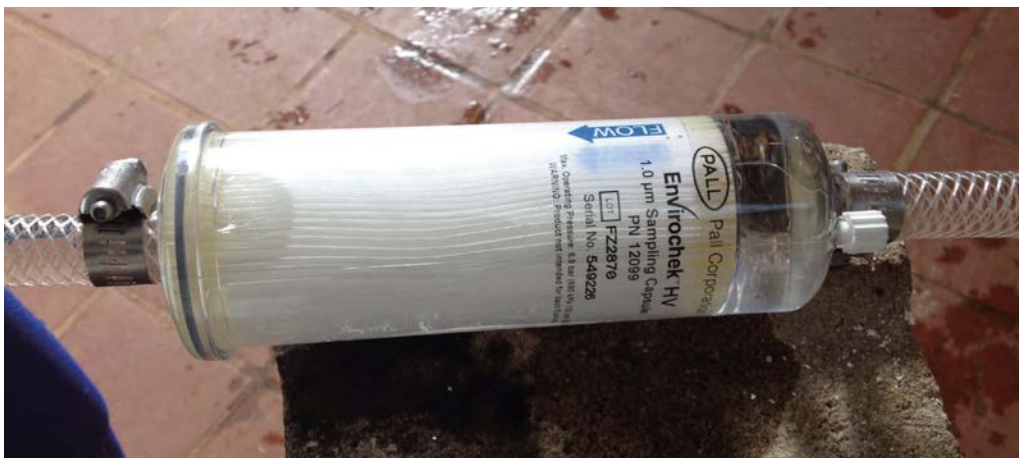
The filter used to look for Cryptosporidium
